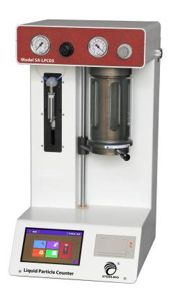
The **Sterilbio Model SA-LPC05** liquid particle counting system provides immediate particle concentration data for low and high viscosity fluids. Using a light blocking sensor, the **Sterilbio Model SA-LPC05** system pressurizes fluid in a chamber for precise volumetric sampling of hydraulic fluids.
